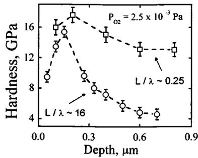
FIG. 1. Hardness vs depth obtained at two extreme conditions of total chamber pressure as a function of  $L/\lambda$  (average number of collisions). The experiments are performed at  $P_{O_2} = 2.5 \times 10^{-3}$  Pa. The lines are a guide for the eyes.
