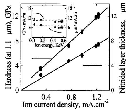
FIG. 7. Linear dependence of the hardness (at constant depth) and nitrated layer thickness vs ion current density (at the surface sample). Inset: hardness and thickness normalized to ion density vs ion energy in (GPa/mA cm<sup>-2</sup>) and ( $\mu\text{m}/\text{mA cm}^{-2}$ ), respectively.
