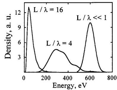
FIG. 5. Ion energy distributions at different  $L/\lambda$  ratios using an inelastic scattering model.
