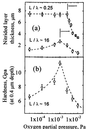
FIG. 2. (a) Nitrided layer thickness (depth penetration) vs oxygen partial pressure obtained at two extreme conditions of  $L/\lambda$  (average number of collisions); (b) hardness (at constant depth) vs oxygen partial pressure ( $L/\lambda \sim 16$ ). The lines are a guide for the eyes.
