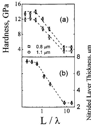
FIG. 4. (a): Hardness vs  $L/\lambda$  at two different depths. (b) Nitrided layer thickness vs  $L/\lambda$ . The lines are a guide for the eyes.
