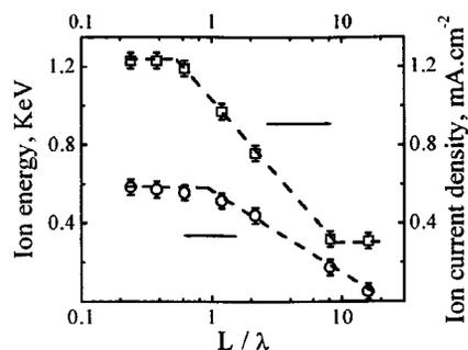
FIG. 6. Mean ion energy and ion current density at the sample surface vs  $L/\lambda$ . The lines are a guide for the eyes.
