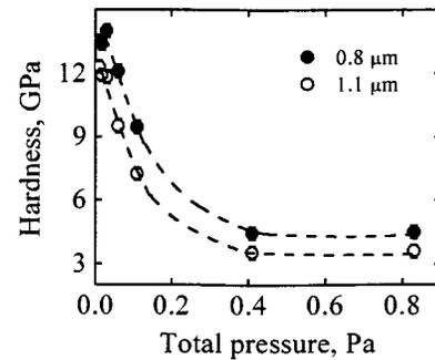
FIG. 3. Hardness vs total chamber pressure at two different depths. The lines are a guide for the eyes.
