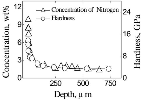
Figure 3. Concentration and hardness curves vs depth for the sample IB3.
