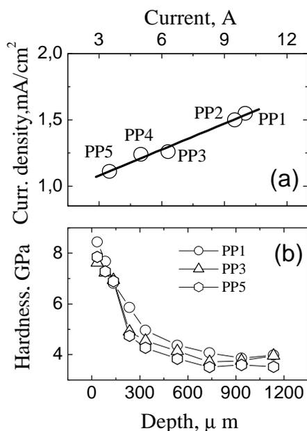
Figure 5. (a) Left axis: effective current density during plasma pulsed nitriding using the correlation obtained from figure 3 as a function of depth. Top axis: nominal current in the plasma pulse experiments; (b) Hardness vs. depth during the pulsed plasma nitriding. For the sake of clarity, only a selected group of curves are displayed in this panel.
