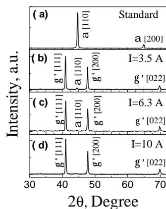
Figure 2. Diffraction patterns of the AISI 4140 samples treated by pulsed plasma. Only the  $\gamma'$  phase is observed.
