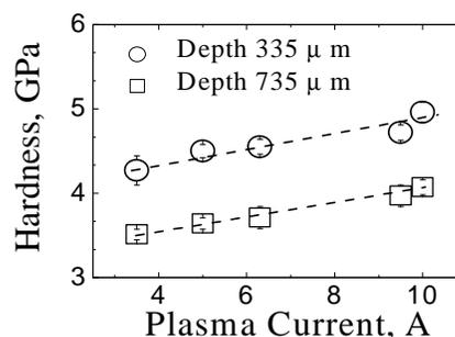
Figure 6. Hardness vs plasma current, for  $\sim 335 \mu\text{m}$  and  $735 \mu\text{m}$  depth corresponding to the plasma pulsed samples.
