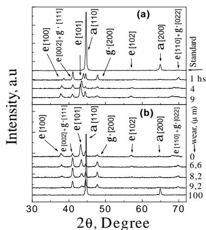
Figure 1. a) Diffraction patterns of as received (standard) and nitrided samples at different treatment times (see Table I). b) Examples of X-rays pattern for the IB3 sample at different depths. The wear thicknesses are indicated. The curves are arbitrarily shifted.
