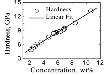
Figure 4. Hardness vs nitrogen concentration curve displaying the proportionality between these quantities.
